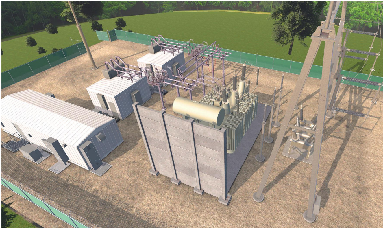
A 3-D generated digital twin. A digital twin, or a 3-D virtual representation of a substation, is a highly accurate tool for finding line of sight. Graphic by POWER Engineers, Inc.
